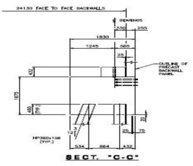
Embedment into concrete is considered as restraint in function of stiffness of the pile and pile cap. Moments are covered in pile-caps.
